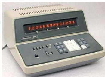
Casio releases the world's first programmable electronic desk-top calculators with program (AL-1000 series) (1967)
